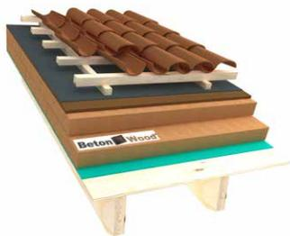
Ecological roof systems for thermo-acoustic insulation with Therm wood fiber density 160 kg/m<sup>3</sup> and Bitumfiber wood fiber density 280 kg/m<sup>3</sup> on matchboarding
