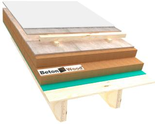
Complete reflective ventilated system for thermo-acoustic insulation with cement bonded particle boards and wood fiber panels
