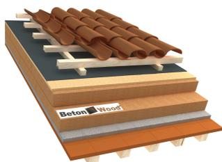
Ecological roof systems for thermo-acoustic insulation with Therm wood fiber density 160 kg/m<sup>3</sup> and Isorel wood fiber density 230 kg/m<sup>3</sup> on terracotta tiles
