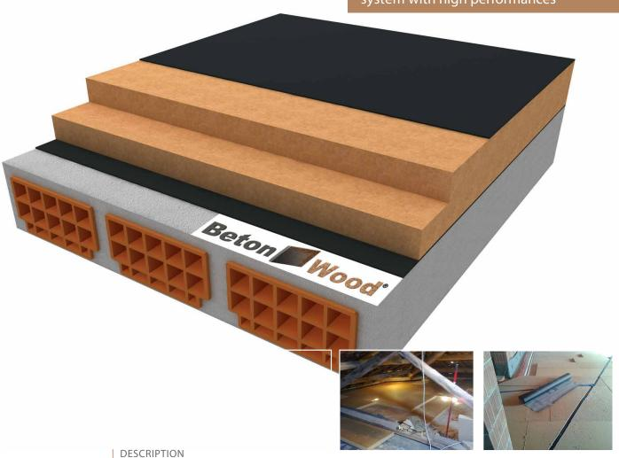
Complete screed system on concrete or cement ground (new or existing) with dry building system which consists in a double layer of rigid wood fiber panels with medium density (160kg/m³)
